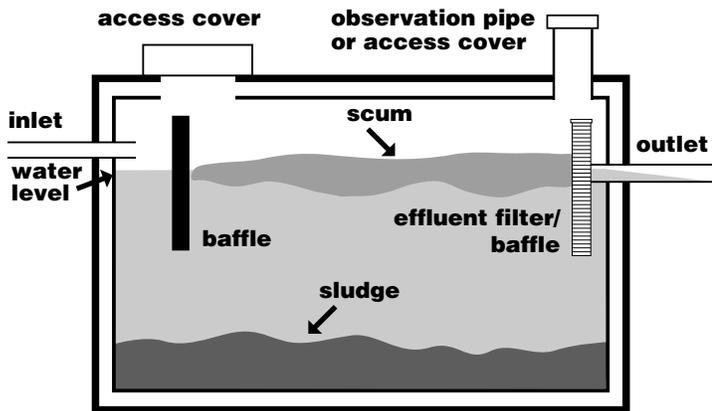
Residential septic systems include the household plumbing, a septic tank, and a drainfield (in-ground, at-grade, mound, or seepage pit).
